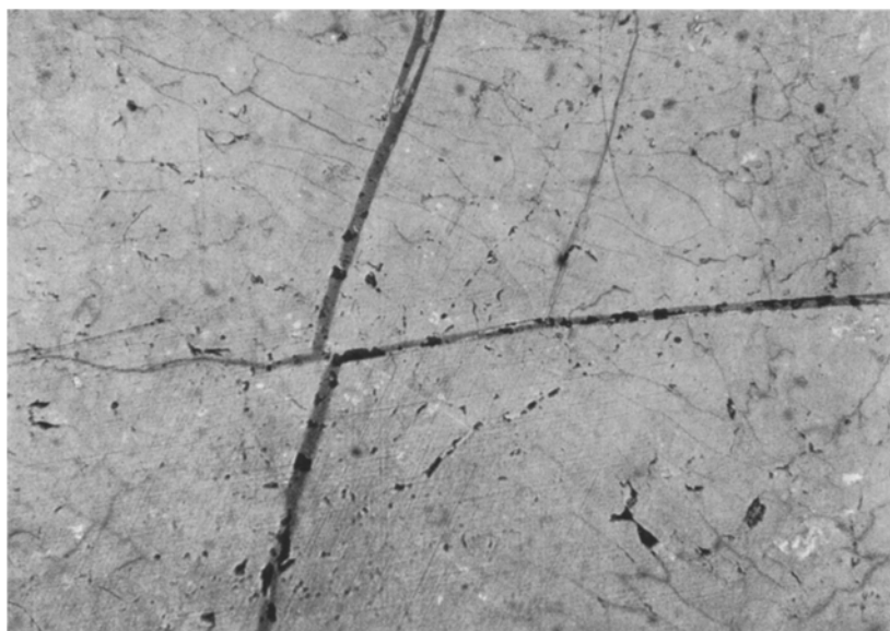
Fig. 1. Veinlets of quartz and crandallite containing some Sr, Ba and rare earths cutting the pandaïte matrix (50 ×)
